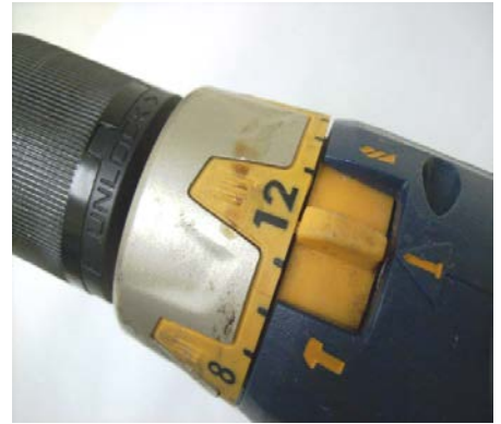
3. Set to 'screw' mode, adjust drill torque clutch setting to achieve 30 to 36in-lbs.
